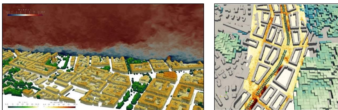
Fig.1: Flow modelling in urban boulevard in Helsinki: 1-instantaneous wind field; 2- dispersion of traffic emissions on and around a planned city boulevard 1 (Kurppa et al. 2019 - Finnish Meteorological Institute and Helsinki University).
