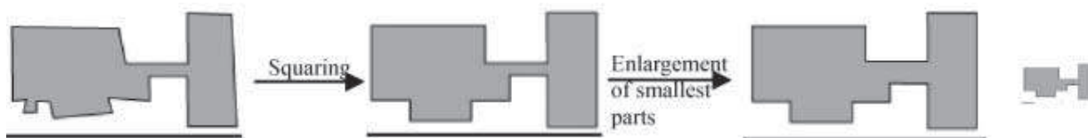
Figure 7: Squaring and selective enlargement leading to changes in constraint values (adapted from Ruas 1999).
