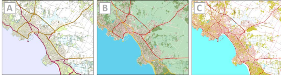
Figure 1. United Kingdom (paper map) (A), Netherlands (digital map) (B) and Finland (digital map) (C) symbol specifications applied to an IGN dataset (Renard 2008).
