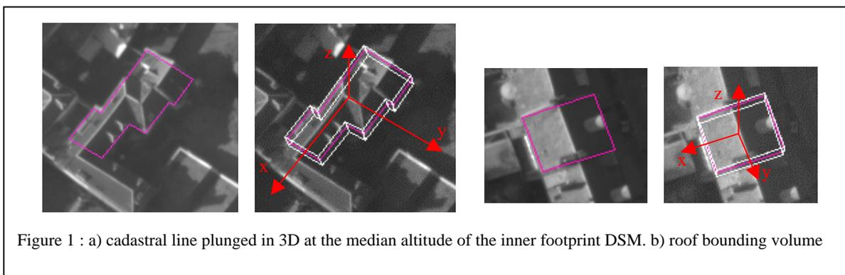
Figure 1 : a) cadastral line plunged in 3D at the median altitude of the inner footprint DSM. b) roof bounding volume
