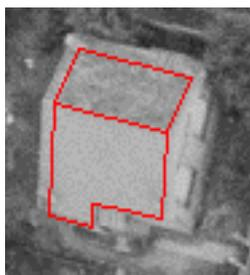
Figure 8 : roof surface generated with the hough transform
