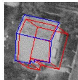
Figure 10 : Roof surface plus the volume defined by the vertical walls
