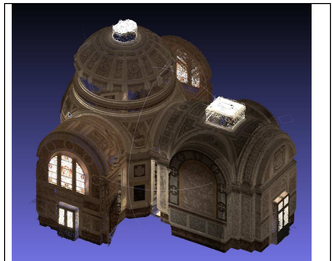
Figure 1. Modelisation of chapelle imperiale, ajaccio. The figure 1 represents a modelization of a chapel, realized with around a hundred images acquired with D5-Mark2 and 15mm fish-eye. This modelization was made by a trainee of MAP Gamsau while developing the interface described in (Godet 2010).
