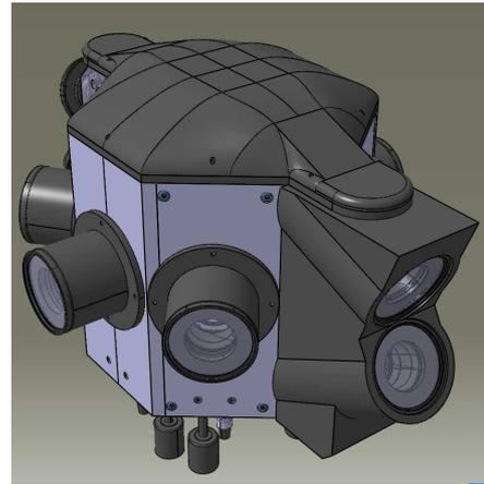
Figure 1: (on the left) the STEREOPOLIS II mobile mapping system. (on the right) the design of the panoramic head with 10 full HD cameras
