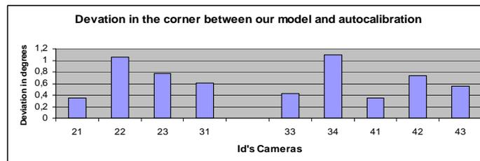
Figure 3: Deviation on corner between our calibration and auto-calibration
