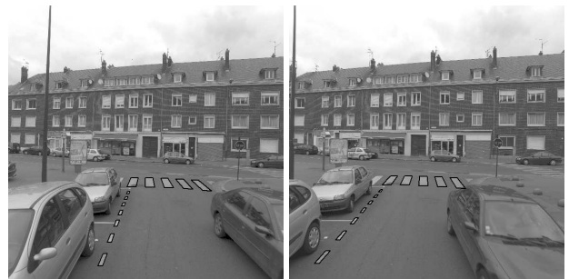
Figure 6: The reconstructed zebra-crossing and dashed-line.
