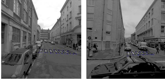
(a) 7 bands out of 7 are detected and correctly reconstructed (b) 6 bands out of 6 are detected. 1 band is not correctly reconstructed due to non-flat band
