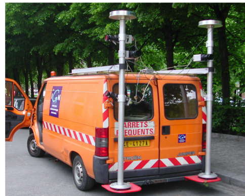
Figure 1. The Stereopolis Mobile Mapping System
