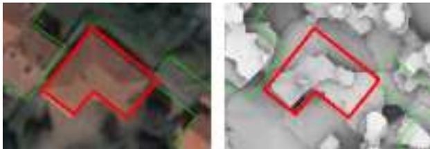
Figure 1. Example of a building (true orthophoto and shaded DEM) : there are 2 triangular facets.
